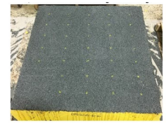
f) Specimen after two coats of epoxy application
