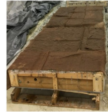
b) Moist curing with wet burlap
