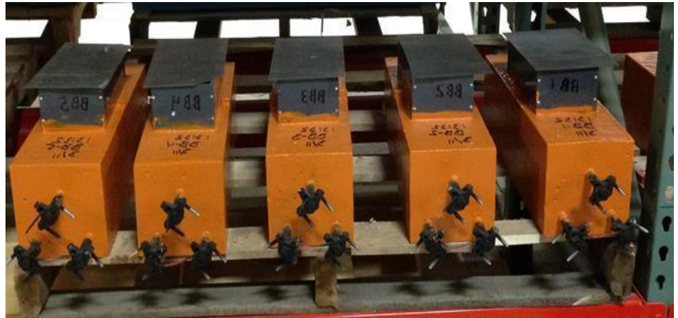
Flexural corrosion beams with cracks under testing.
